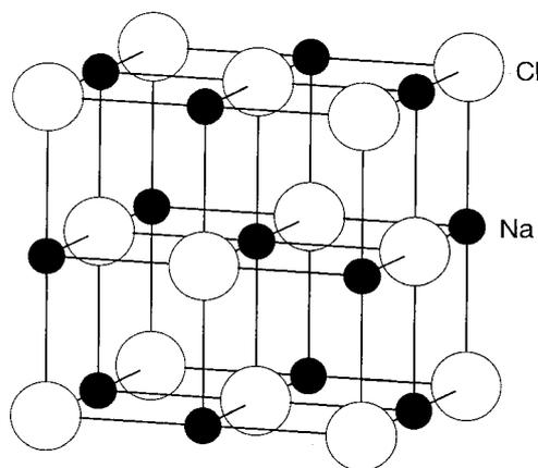
**Fig. 2.7** Rock-salt structure.
