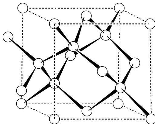
**Fig. 4.5** Structure of diamond.
