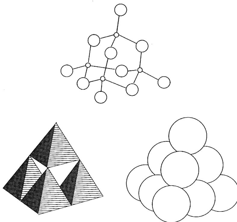
**Fig. 2.12** Three expressions for the structure of  $P_4O_{10}$ .
