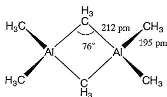
**Fig. 5.2** Structure of trimethylaluminum.
