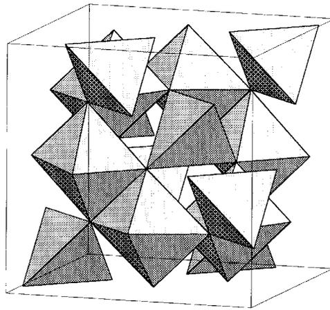
**Fig. 4.15** Spinel structure.
