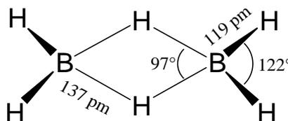
**Fig. 4.2** Structure of diborane.
