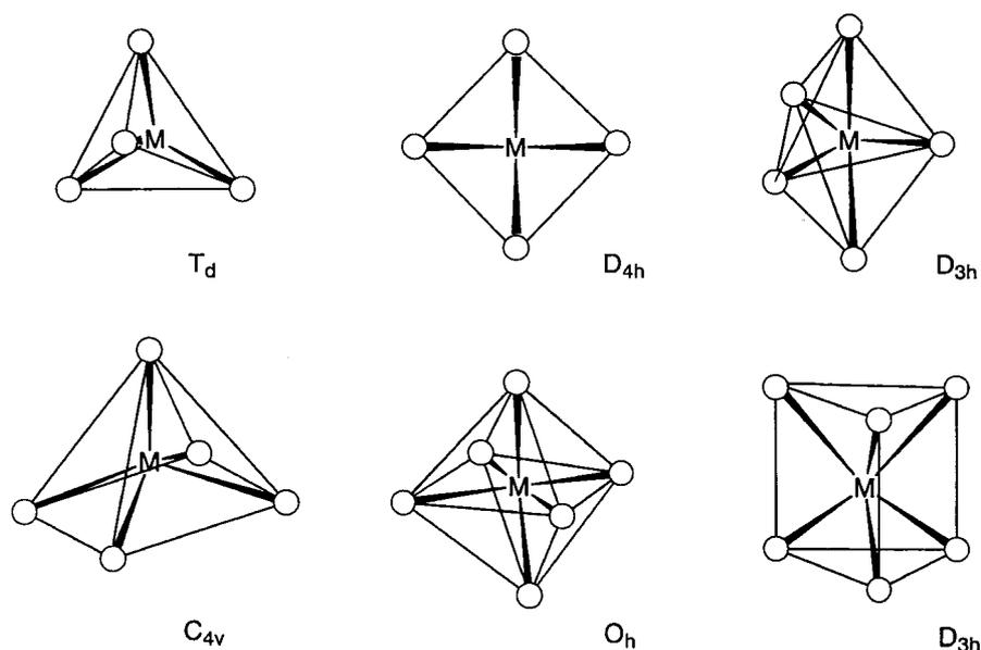
**Fig. 6.1** Structure of 4 ~ 6 coordination.
